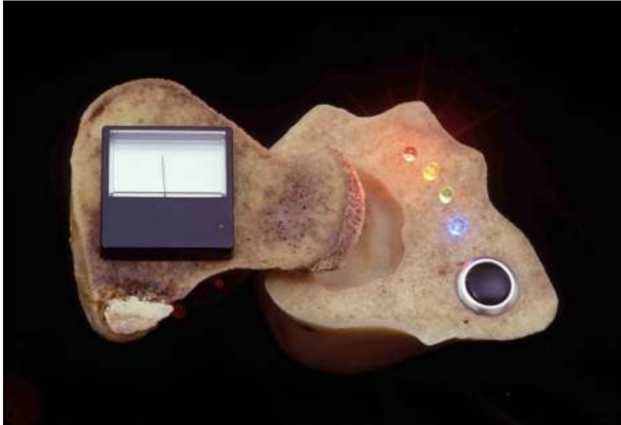
Handheld interactive device based on BasicStamp platform
